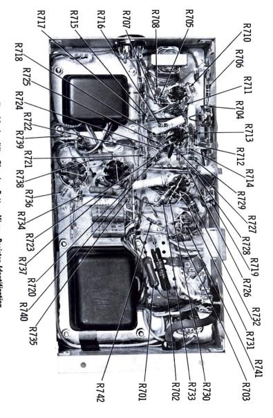
Fig. 22. Amplifier Chassis—Bottom View—Resistor Identification.
