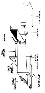
Fig. 8. Lower Keyboard—Key Construction.
