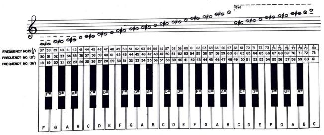
\* FREQUENCY AT OUTPUT OF DOUBLER CIRCUITRY Fig. 1. Notes on Upper Keyboard.
